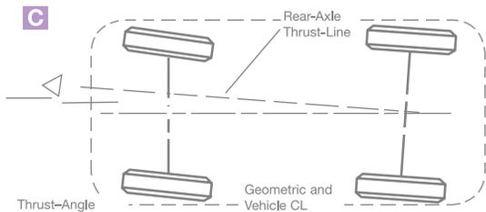
If the rear axle or wheels are toed to one side **C**, the thrust line will not match up with the center line and the vehicle will pull—in this case—to the left.
