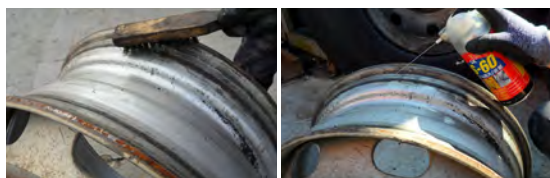
<Retirez la corrosion>
